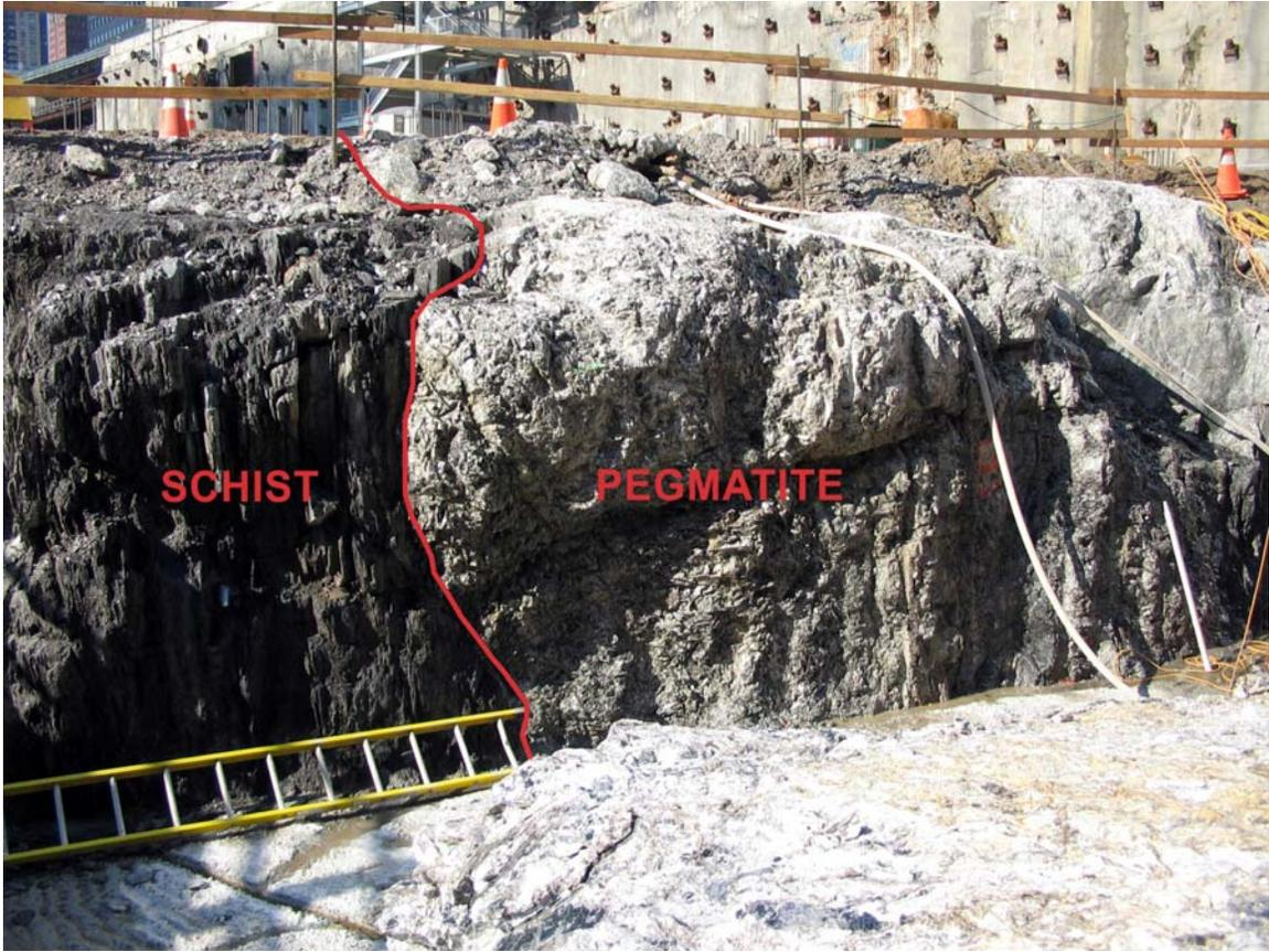
**Figure 5** – Pegmatite intrusive (seen on the right) into schistose rock in the NW corner of the WTC site. The pegmatite is essentially the same in both the NW and SE corners of the site. (Image by C. J. Moss.)
