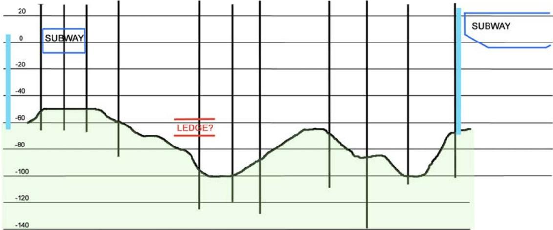
**Figure 6** – Cross-section through the depressions in the east bathtub, facing north. Red lines show the location of either a ledge of bedrock or an 11 foot thick pegmatite boulder. Location of cross-section is shown in Figure 7. Elevation 0' is equal to El +2.653' on USGS Mean Sea Level Datum at Sandy Hook, NJ (1929 NGVD).
