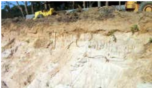
Figure 2 - Till exposure (dark tan) located above outwash sediments (light tan) at the new East Moriches K-4 Elementary School. Stick is one meter in length. South is to the right of the figure.
